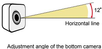
Adjustment angle of the bottom camera
